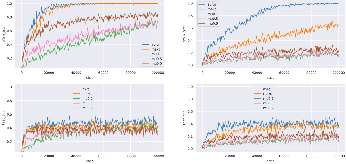
Figure 4: CIFAR100: Training (top) and test (bottom) accuracies for the Adagrad-like ( \mu \in (0.1, 0.5, 0.9) ), maxgi and avrgi variants with \gamma = 5 \cdot 10^{-4} (left) and \gamma = 5 \cdot 10^{-5} (right) on the resnet18 architecture
